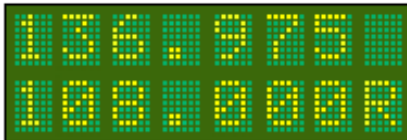
Monitor Mode Receiving on STANDBY frequency
