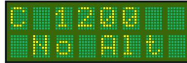
The “No Alt” diagnostic means that the T2000SFL transponder cannot interpret the code on its parallel inputs (*the ten wires that come from the altitude encoder*) as a valid altitude. The fact that “No Alt” is displayed means that the main microprocessor is working. It simply doesn’t understand what it is seeing. There are a few reasons why this may happen.
